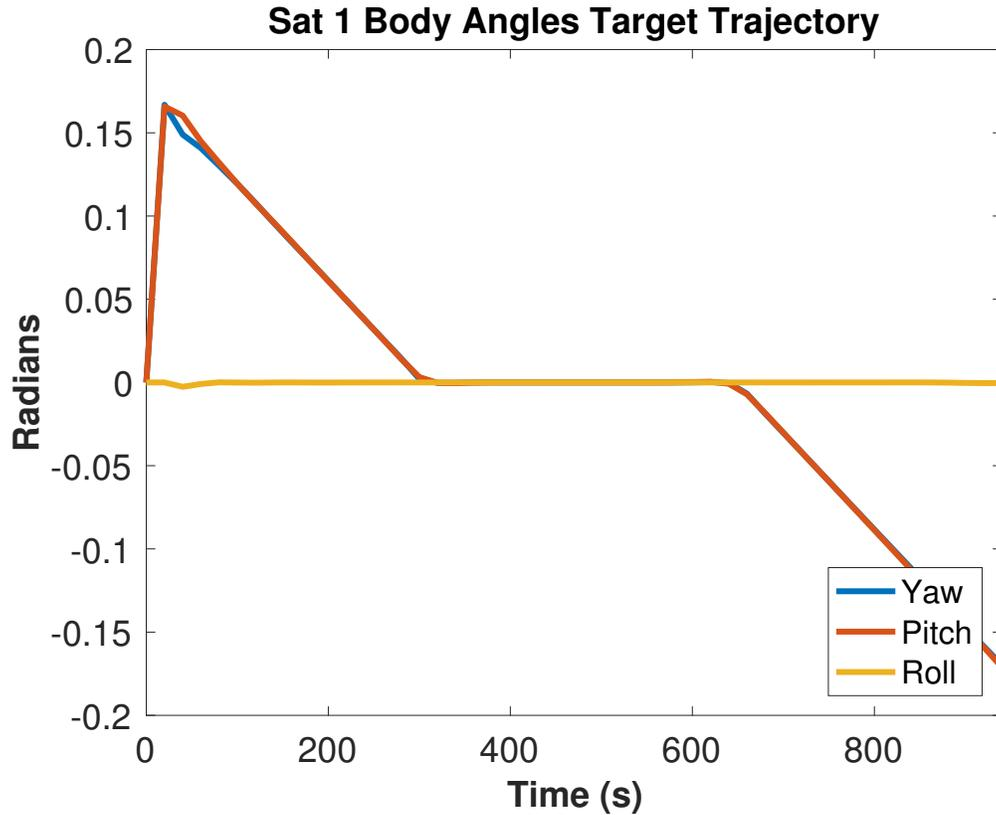
Figure 6.3: Plot of the emitter satellite's body angles as part of the target trajectory
